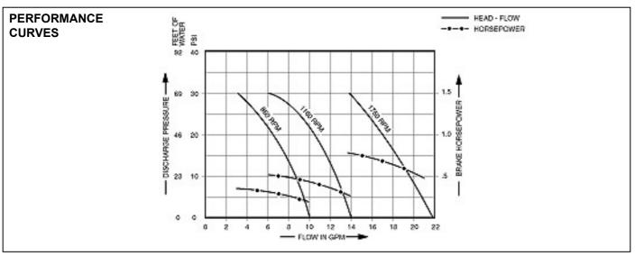
NOTE: Curves show approximate head-flow for new pumps with neoprene impeller pumping water. Capacities should be reduced approximately 10% with nitrile, viton and EPDM impellers. Consult factory for specific performance information.
