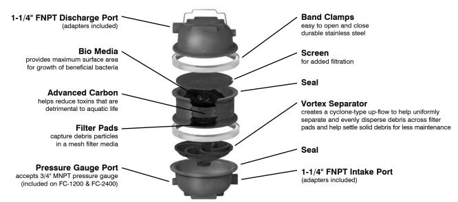
The BioVort<sup>™</sup> filter combines biological and mechanical filtration to provide clearer water, a healthier environment, and less maintenance in a pond environment.
