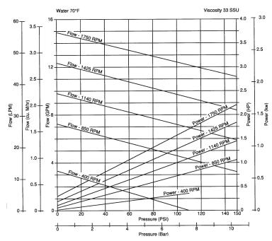
Notes: For continuous service: Plastic / Plastic gear combinations are limited to 50 psi. Metal / Plastic gear combinations are limited to 100 psi. Metal/Metal gear combinations are limited to 150 psi.
