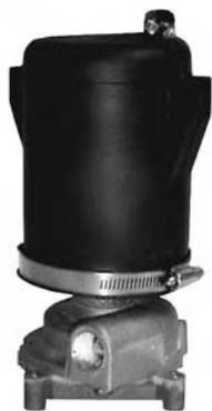
**CP-5009 Installation:** CP-5009 has a 1" NPT inlet and may be installed into a rigid 1" piping system. Do not install CP-5009 directly on top of a 1" seacock. The rubber boot protects the motor, so CP-5009 can be submerged without harm.
