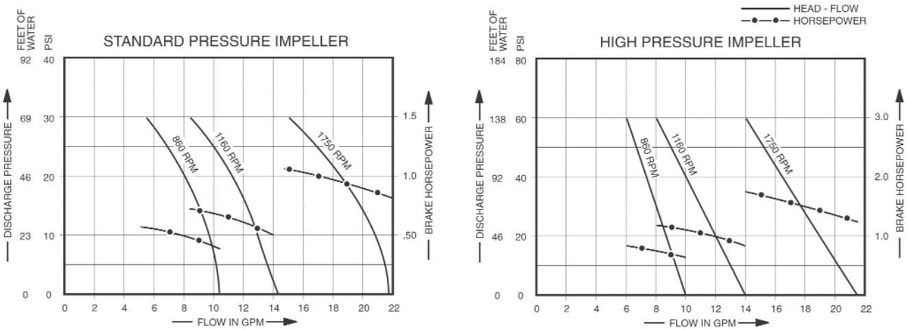
NOTE: Curves show approximate head-flow for new pumps with neoprene impeller pumping water.
