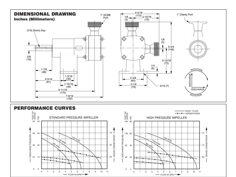
NOTE: Curves show approximate head flow for new pumps with neoprene impeller pumping water. Capacities should be reduced approximately 20% with high pressure EPDM impeller.
