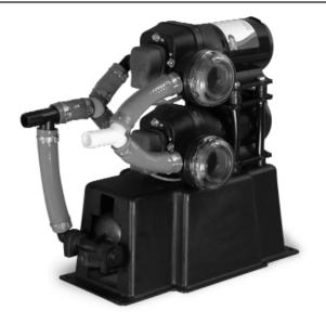
The accumulator tank smooths water flow and reduces on/off cycling of the pump by lessening the variation in pressure. Even flow of water gives better control of hot water temperature especially noticeable with instantaneous gas water heaters and showers. Reduced on/off cycling reduces noise from the pump, water hammer and gives longer pump life.
