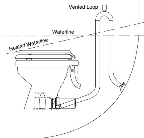
If the toilet is plumbed to an overboard discharge, and is below the vessel's waterline, the discharge plumbing must include a properly positioned vented loop. The vented loop fitting must be secured in a location that remains at least 6-8 inches (15-20 cm) above the waterline at all angles of heel and trim. The maximum discharge head without a notable decrease in pump performance is four feet (1.3 M).
