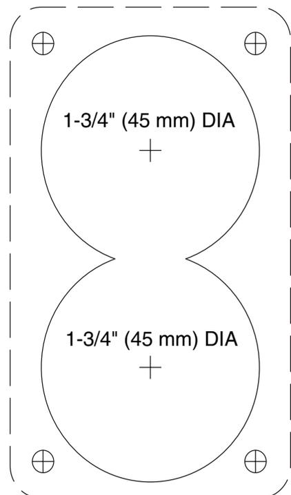
diameter holes (slightly over-lapping) through the selected switch mounting surface per the attached template. Ensure the template is oriented correctly because it is not symmetrical. Also, drill four appropriate sized holes for the fasteners selected to secure the switch panel to its mounting surface.
