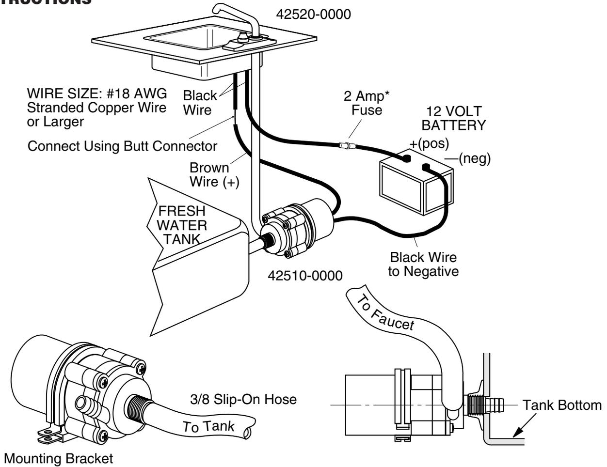
**MOUNTING:** Mount with bracket and connect with slip-on hose below lowest water level or thread into 3/8" bottom tank fitting. Connect 3/8" hose between discharge port of pump and faucet ensuring hose rises continually from pump to faucet.
