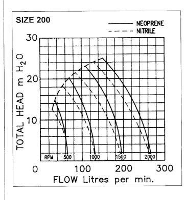
Performance Note Power (watt) figures shown are minimum recommended at pumpshaft.
