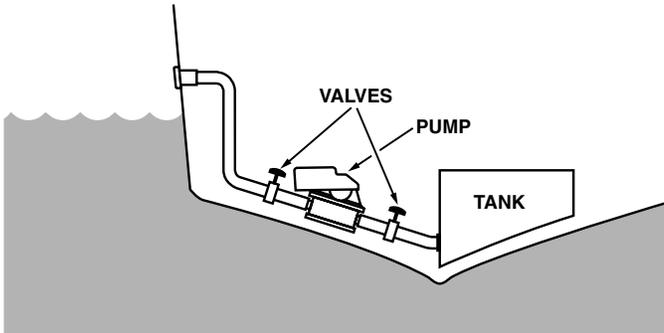
If the waste discharge plumbing can not be connected to a thru-hull positioned above the water line, the discharge plumbing must be fitted with a 1-1/2" vented loop positioned to remain about 8" above the water line at all angles of heel and trim.
