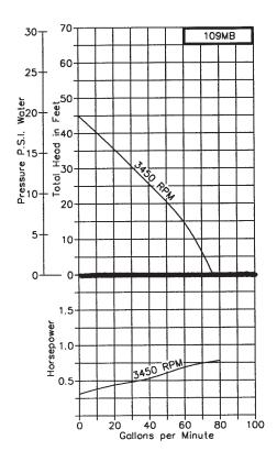
horsepower in direct proportion to the increase in specific gravity. Liquids contaminated with small solids or abrasives can be handled, but a reduction in mechanical seal life must be expected.
