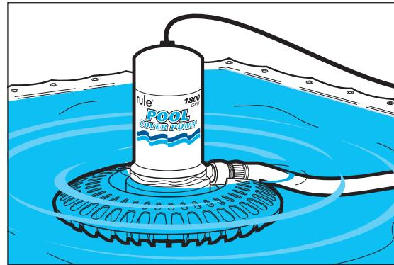
**Note:** Restricting the flow from a Rule pump by using a smaller pipe or hose size (such as a garden hose) does not damage the pump, but will result in a reduction in flow. For maximum flow, use the shortest length of the largest diameter hose available.
